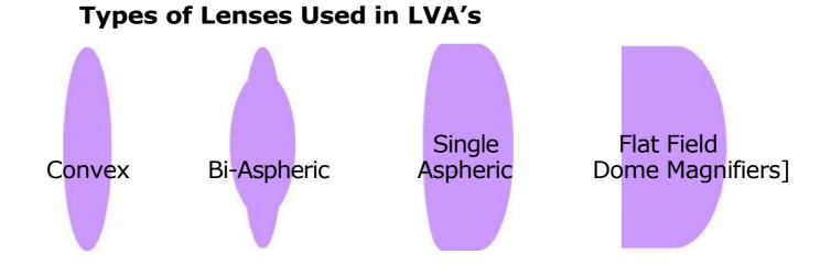
The shapes of some of the lenses illustrated above have been exaggerated to identify the differences more clearly.
